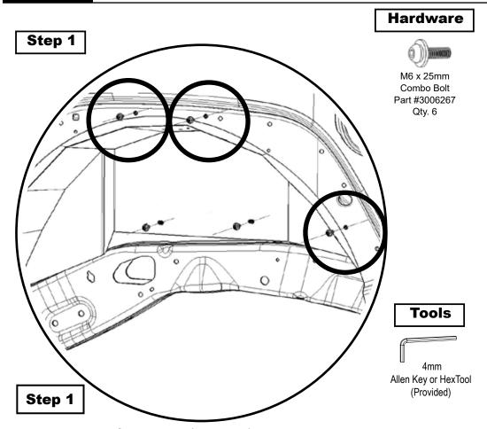
Hand install the Combo bolt (3006267) into the Wheel Well Liners riventnuts by inserting three (3) bolts per side. Make sure to check and lineup body holes with the threaded insert holes in fender liners.
