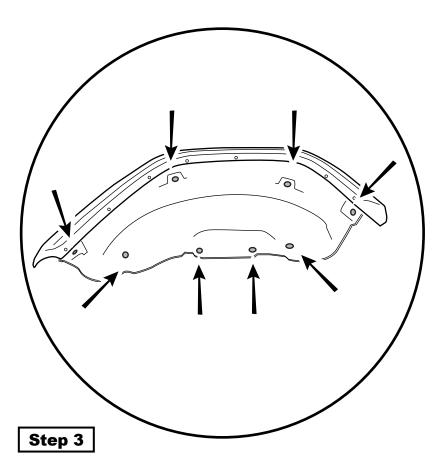
To remove pry up on all the plastic trees that join the liner to the Jeep body.
