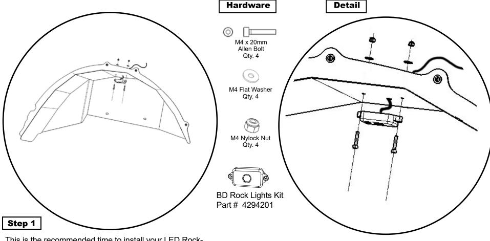
This is the recommended time to install your LED Rocklights and wiring onto the vehicle and wheel well liners, per best practices and per the lighting manufactures instructions.
