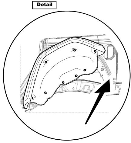
With the inner liner fasteners removed and loose, now you can remove the entire fender. Grab the fender and pull the fender away from the body. It's attached with clips. When pulling it away the clips will probably break. Fasteners will not be reused in this install.
